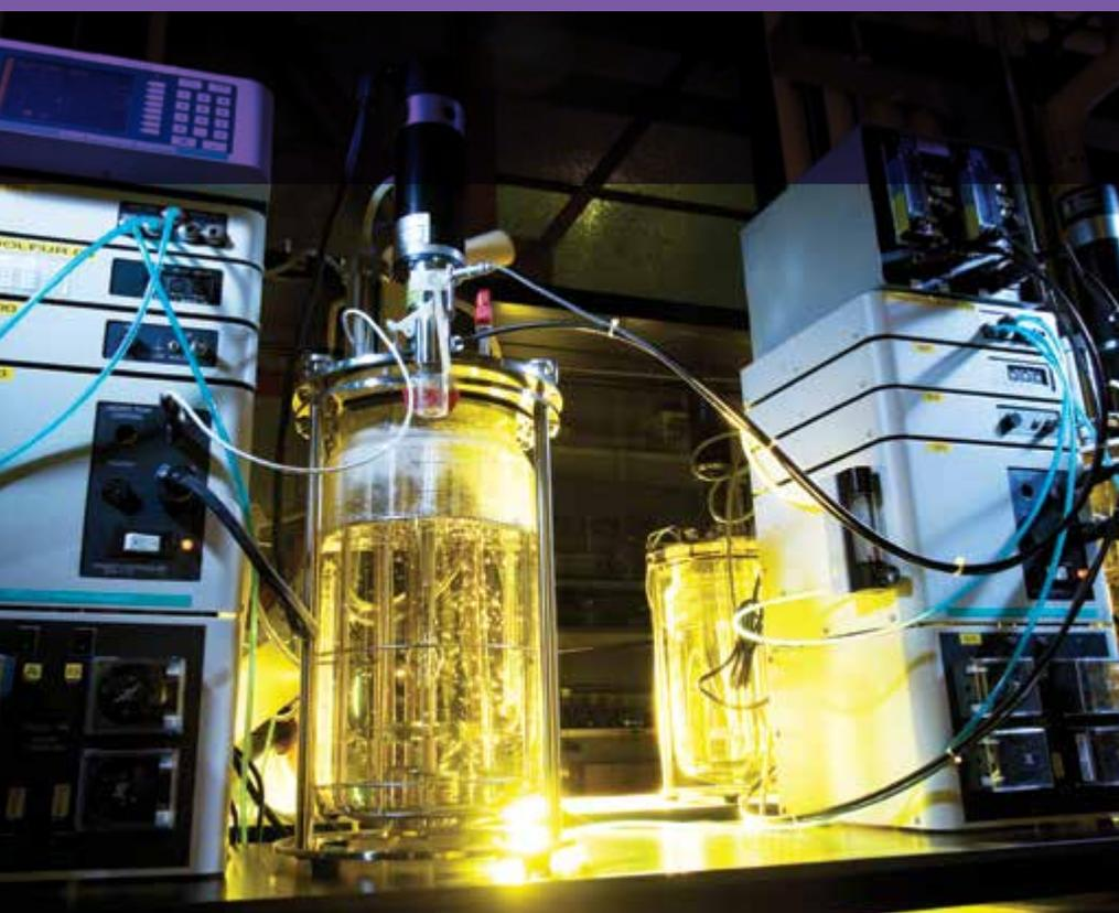
Modular bench-scale bioreactors for accelerated and integrated scale-up process development
