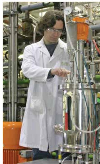
Preparation of a 20 L bioreactor for a microbial fermentation
